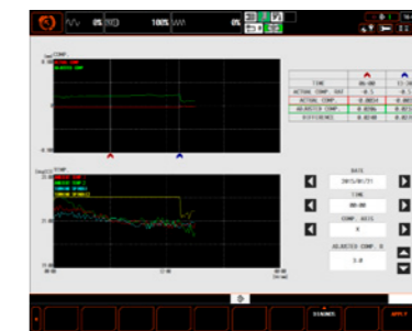
Temperature and compensation are displayed on MAZATROL SmoothG screen. Operator can adjust compensation by looking at the data.
